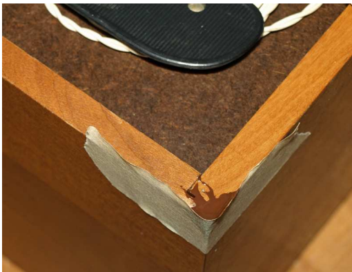
fig 7—corner bash, tape dam and epoxy filler
