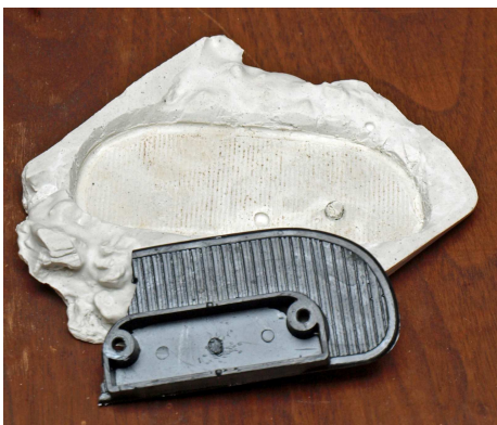
fig 5 – broken cleat & plaster mold
