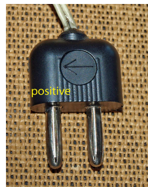
fig 11—speaker plug (against original speaker cloth)
