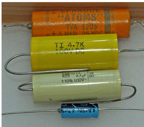
fig 25—Original Sprague electrolytic, Tecate film, ERO film, and new electrolytic
