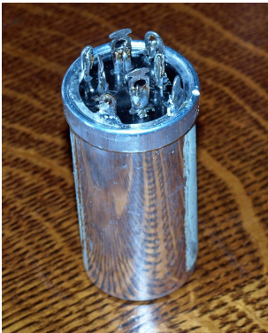
fig 21—completed stuffed can
