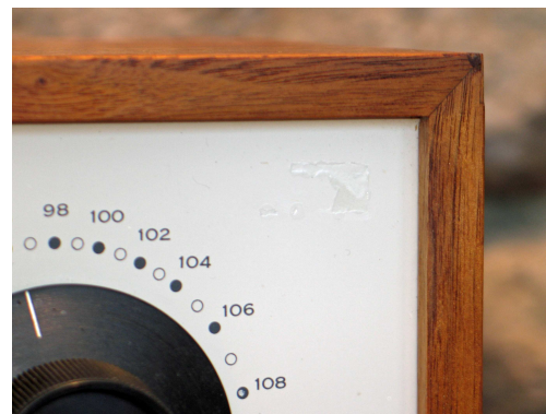
fig 8 – repaired paint chip
