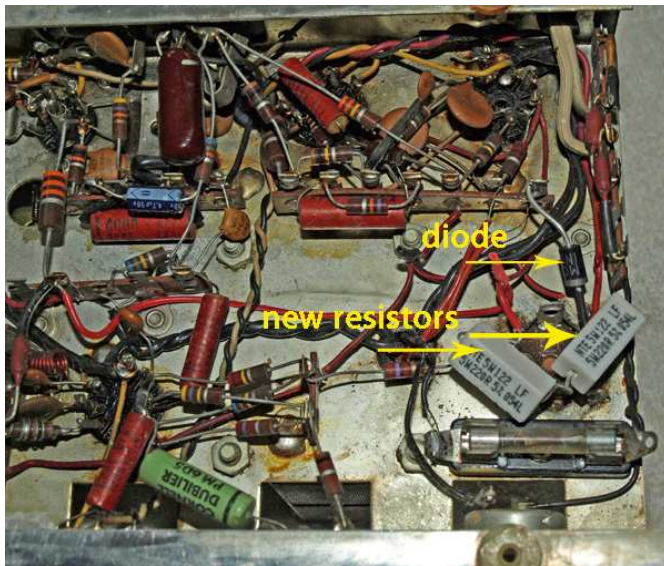
fig 23—new 3-A diode and 5-W resistors
