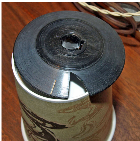
fig 34—broken tuning dial
