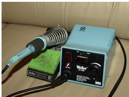
fig 18—pencil type soldering iron
