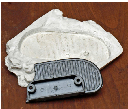
fig 9 – broken cleat & plaster mold
